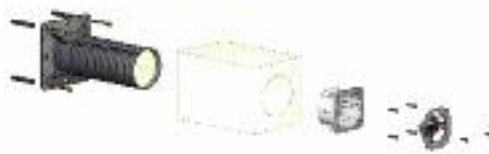
KEZ - installation box into thermal insulation
